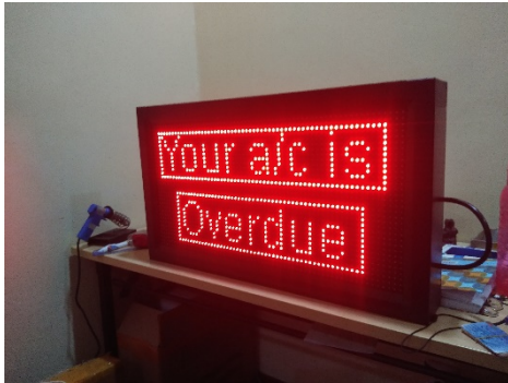
Access Card Blocker (ACB) LED Panel Burn test is in Progress
